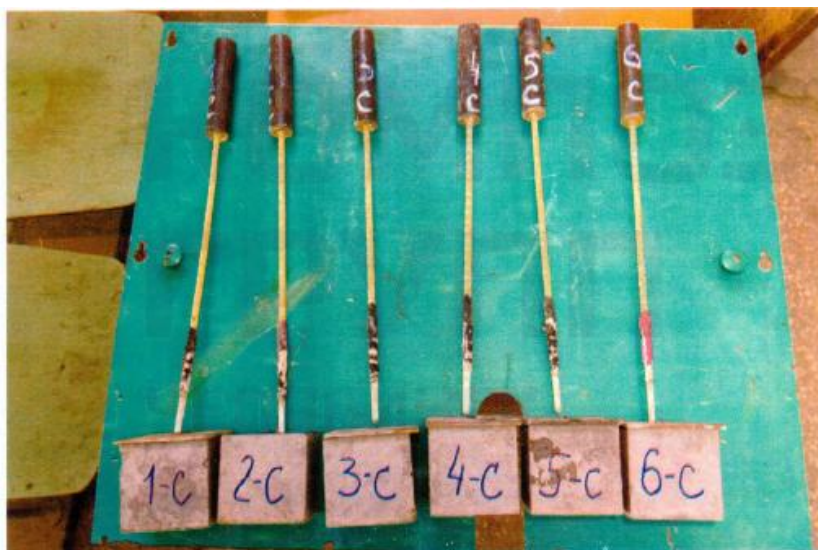
Figure 15 - Composite Fiberglass Reinforcement after Tests of Strength Limit of Concrete Bond after Alkali Exposure
