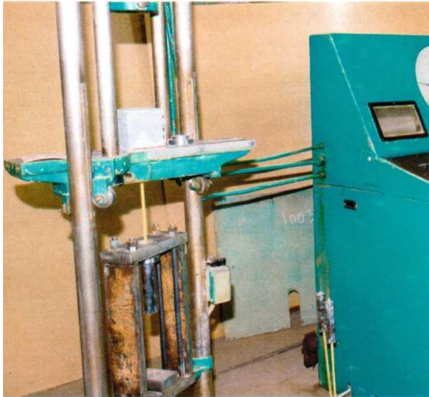
Figure 16 – Course of Testing of Concrete Bond Strength Limit of Fiberglass Rods
