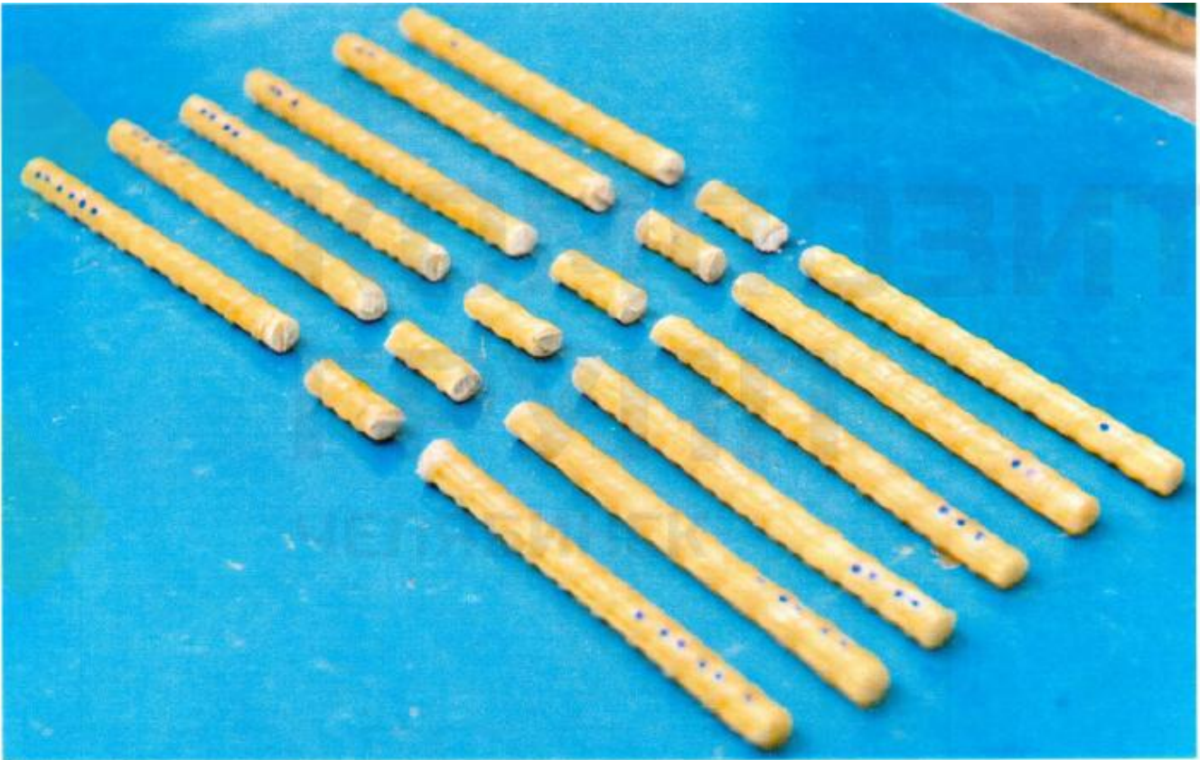
Figure 9 – Composite Fiberglass Reinforcement after Tests for Cross Section
